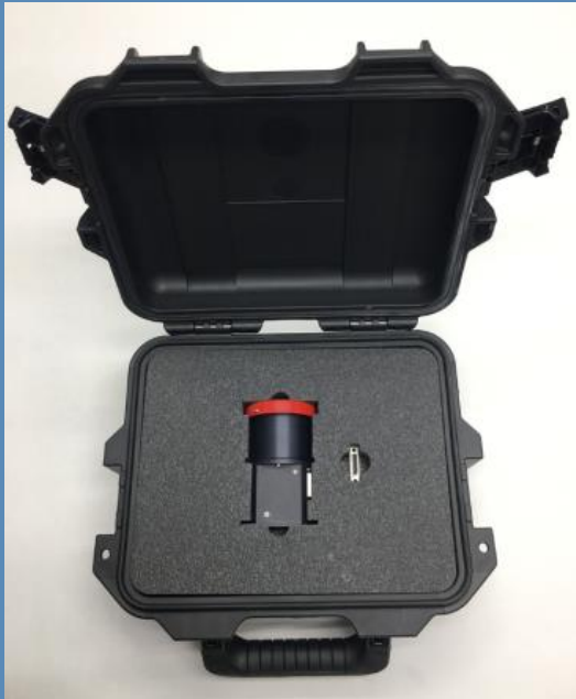
Fig. 2. Nano star tracker AZDK-1 in the transport suitcase
